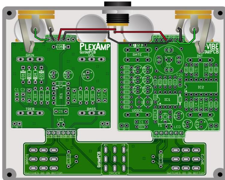
**Order switching is built-in, with pin header connections making wiring a breeze.**
