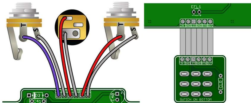
**Easy Wiring Guide – Install the 3PDT switch on the bottom. CLR is the Top.**
